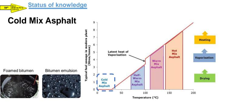
There are still concerns (e.g. high air-void, moisture damage resistance, long curing times required to achieve maximum performance etc) which reduce its widespread usage in asphalt layers
