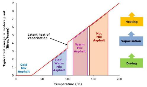
Warm mix asphalt (WMA): produced and mixed at temperatures of 100°C to 140°C
