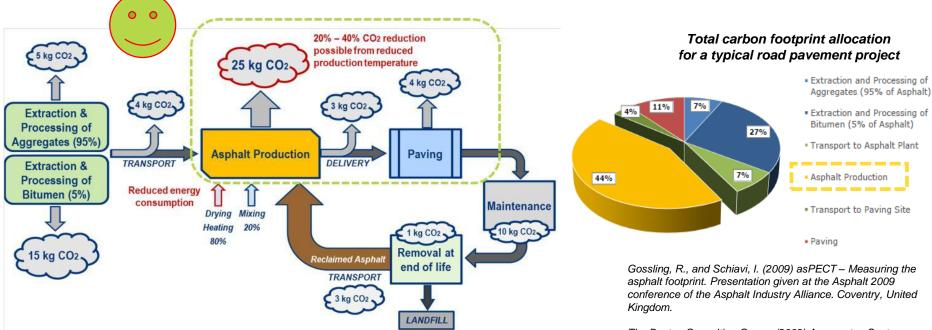
Indicative lifecycle carbon emissions for the production of one ton of asphalt
