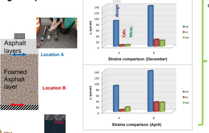
Assessment of strains using Fiber Optic Sensors
