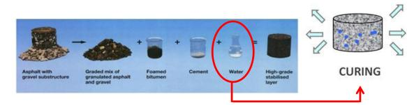
Discharge of water from compacted material due to:
