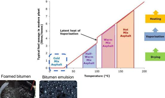
□ Bitumen emulsions (less frequently foamed bitumen) can be mixed with aggregates in ambient conditions to produce cold mix asphalt
