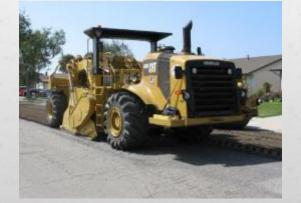
Improves existing materials in-place to provide greater structural support and reduction of imported material.
