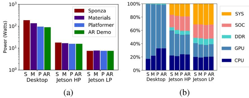
**FIGURE 5.** (a) Total power (note log scale) and (b) relative contribution to power by different hardware units for ILLIXR running each application on each hardware platform. S = Sponza, M = Materials, P = Platformer, and AR = AR Demo. SoC power includes on-chip microcontrollers but excludes CPU and GPU power. Sys power includes display, storage, and I/O.
