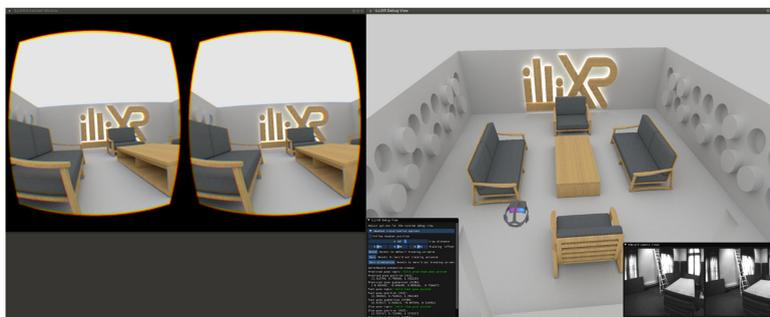
**FIGURE 3.** Left: Stereoscopic images presented to the user. Right: Third-person debug view showing the virtual environment and the pose of the headset within it. The debug view also shows the tracking camera's stereo images on the bottom right and detailed pose information on the bottom left.
