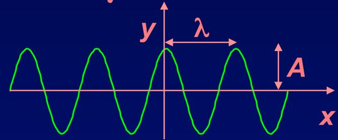
For a wave on a string, each point on the wave oscillates in the  $y$  direction with simple harmonic motion of angular frequency  $\omega$ .
