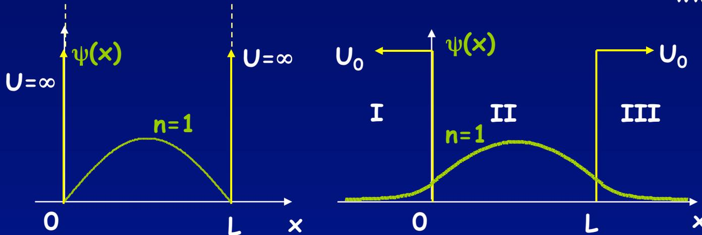
The wavelength in the finite well is longer, because it is not required to go to zero at  $x = 0$  and  $x = L$  (it “leaks” out a little). Thus, the momentum  $p = h/\lambda$  is smaller, and so is the energy. That’s true in general; the less one confines an object, the lower its energy can be - a consequence of the Heisenberg Uncertainty Principle.
