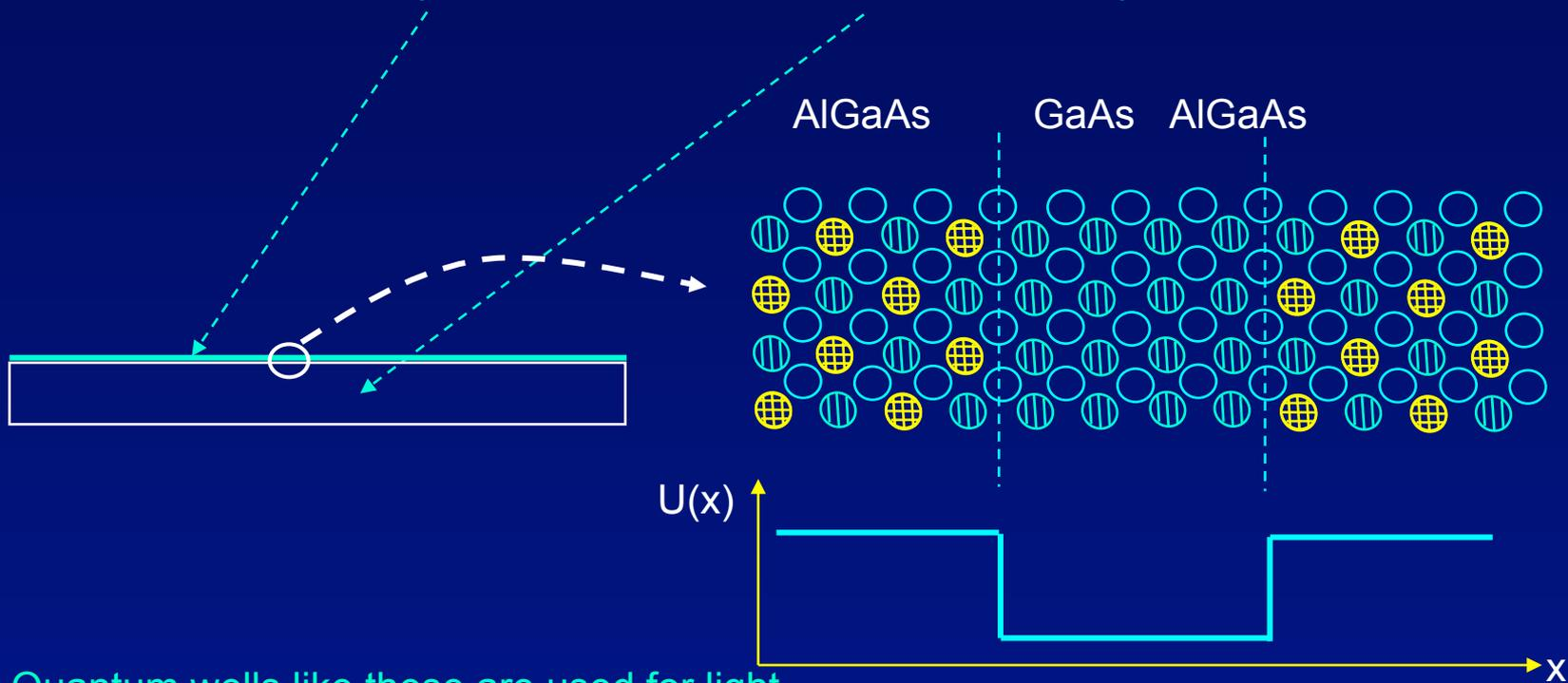
Quantum wells like these are used for light emitting diodes and laser diodes, such as the ones in your CD player.
