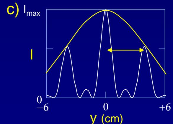
**Interference spacing doubles. Diffraction profile is unchanged.**
