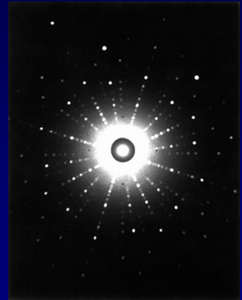
Diffraction pattern from single crystal of Nd 2 CuO 4
