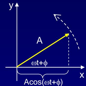
It is conventional to draw one phasor horizontal. Because the phasors are rotating, this merely means we are looking at them at a particular time.
