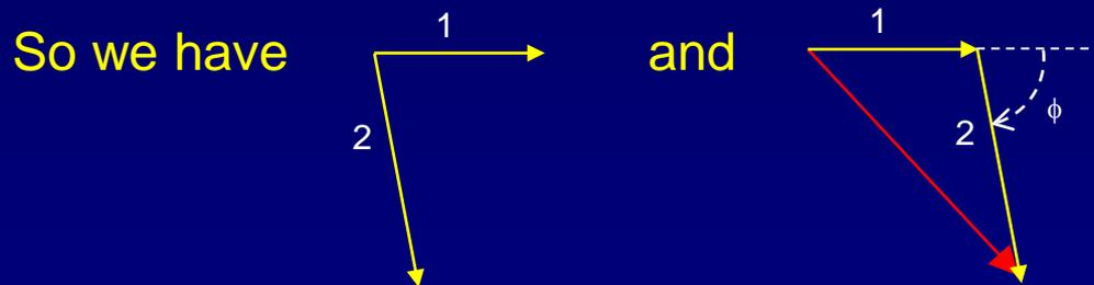
Note that the algebraic solution we wrote before does not apply here, because the amplitudes aren't equal. You can use some trigonometry to calculate the length of the third side of the triangle.
