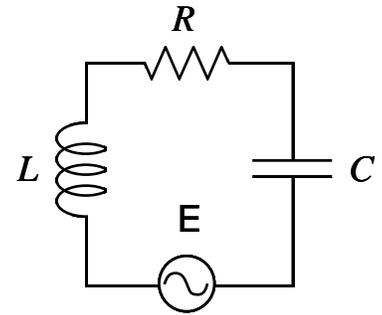
$$\begin{aligned} L &= 40 \text{ mH} & f &= 50 \text{ Hz} \\ C &= 2.5 \text{ mF} & I_{\max} &= 0.5 \text{ A} \\ R &= 15 \Omega \end{aligned}$$
