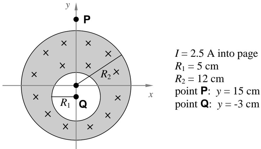
(a) Calculate the magnetic field at the point **P** on the  $y$  axis.
