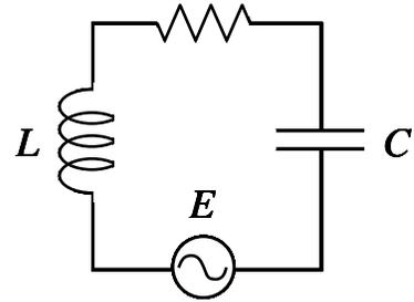
$$\begin{aligned} R &= 200 \, \Omega \\ L &= 40 \, \text{mH} \\ C &= 0.20 \, \mu\text{F} \\ E_{\text{rms}} &= 120 \, \text{V} \\ \omega &= 10^4 \, \text{rad/sec} \end{aligned}$$
