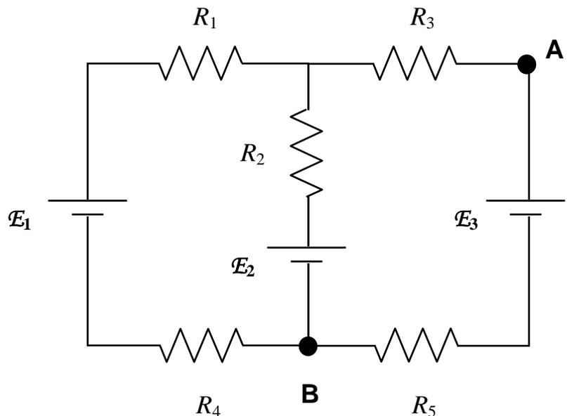
(a) Find the **current  $I_3$**  through resistor  $R_3$ .
