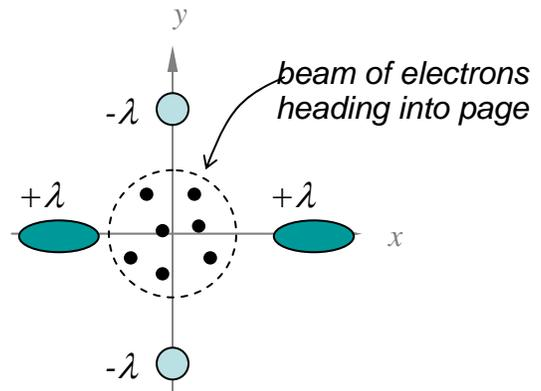
(d) The cathode ray tube (CRT) in a TV monitor contains a beam of electrons directed towards a fluorescent screen. The screen lights up where the beam hits it. If you were an electrical engineer designing such a CRT, why might you find it useful to pass the electron beam through a quadrupole before it hits the screen? (A little hint: quadrupoles are usually used in *pairs* ... can you figure out why?)
