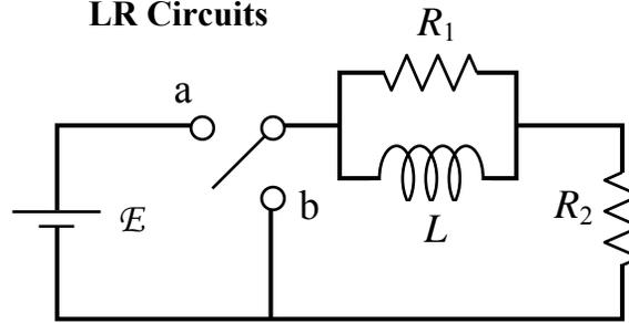
$$\begin{aligned}\mathcal{E} &= 10 \text{ V} \\ L &= 15 \text{ mH} \\ R_1 &= 4 \Omega \\ R_2 &= 6 \Omega\end{aligned}$$
