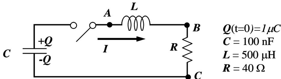
The charge on the capacitor oscillates while dying out as shown below:
