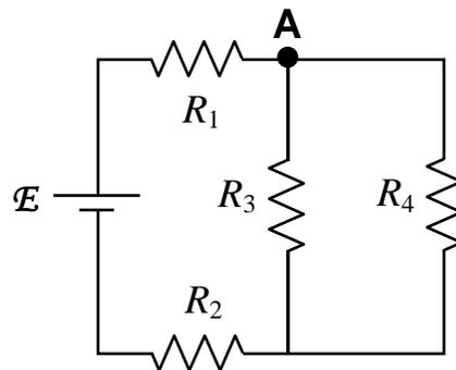
(e) Next, apply *KCL* to every *node* in the circuit. How many nodes are there in this circuit? Write down a *KCL* equation for each one.
