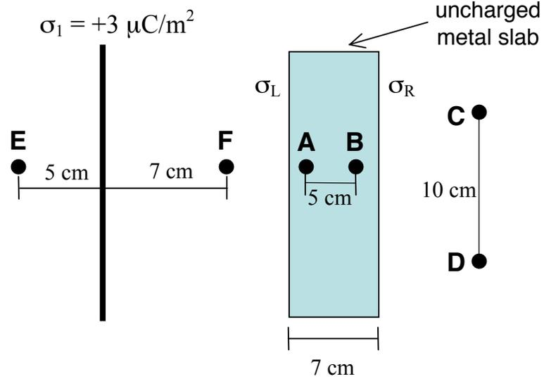
3) What is the potential difference  $V_{AB} = V_B - V_A$  between points **A** and **B** inside the conducting slab? [4]
