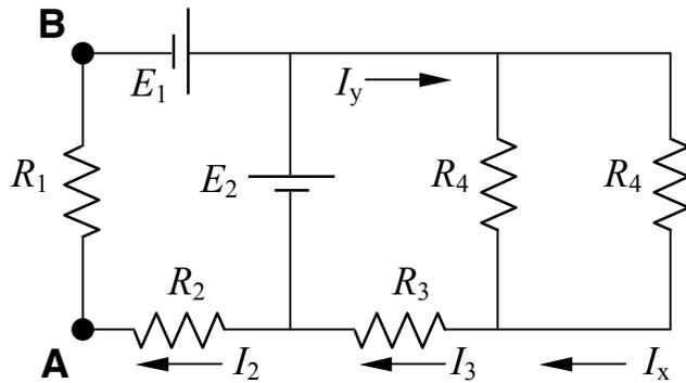
$$\begin{array}{ll} R_1 = 10 \, \Omega & R_2 = 15 \, \Omega \\ R_3 = 30 \, \Omega & R_4 = 25 \, \Omega \\ E_1 = 10 \, \text{V} & E_2 = 30 \, \text{V} \end{array}$$
