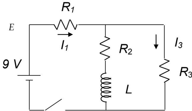
$$\begin{aligned} R_1 &= 30 \, \Omega \\ R_2 &= 100 \, \Omega \\ R_3 &= 150 \, \Omega \\ L &= 0.02 \, \text{H} \end{aligned}$$
