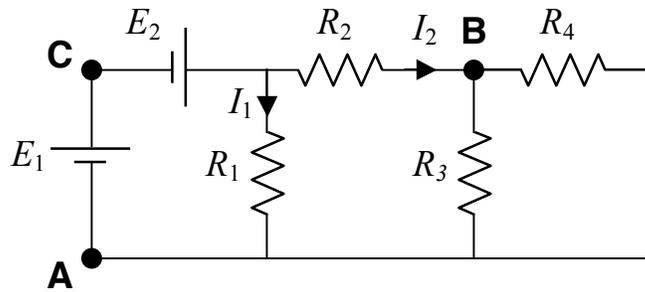
$$\begin{aligned} R_1 &= 60 \, \Omega & R_2 &= 6 \, \Omega \\ R_3 &= 10 \, \Omega & R_4 &= 20 \, \Omega \\ E_1 &= 15 \, \text{V} & E_2 &= 10 \, \text{V} \end{aligned}$$
