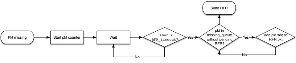
Keep track of state of missing packets in the NF while handling the request for retransmission packets and sequence number of missing packets
