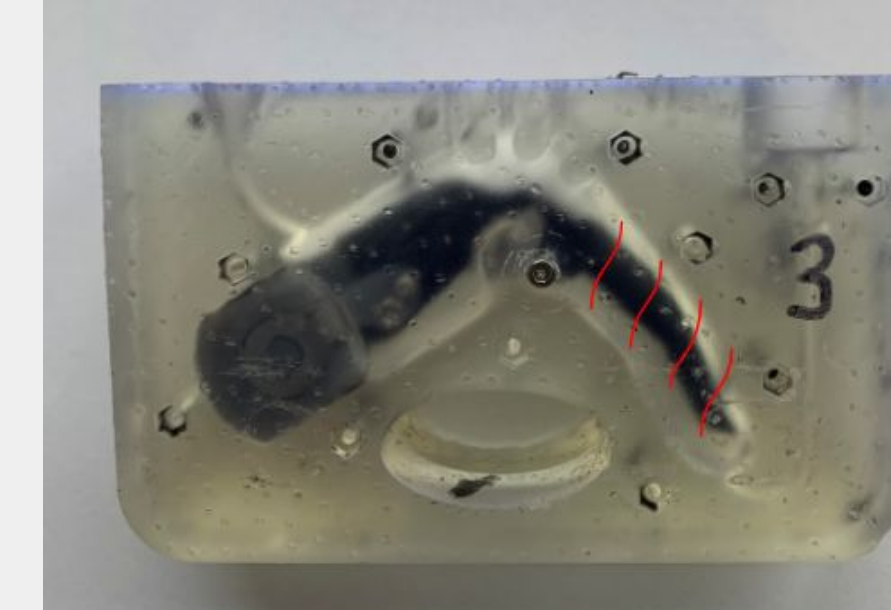
3D Printed finger bone in mold with red lines to simulate wire placement
