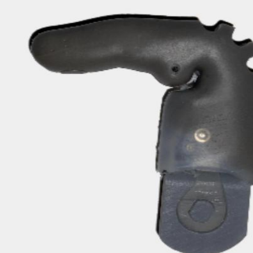
Finger molded with thermal paste and silicone mixture
