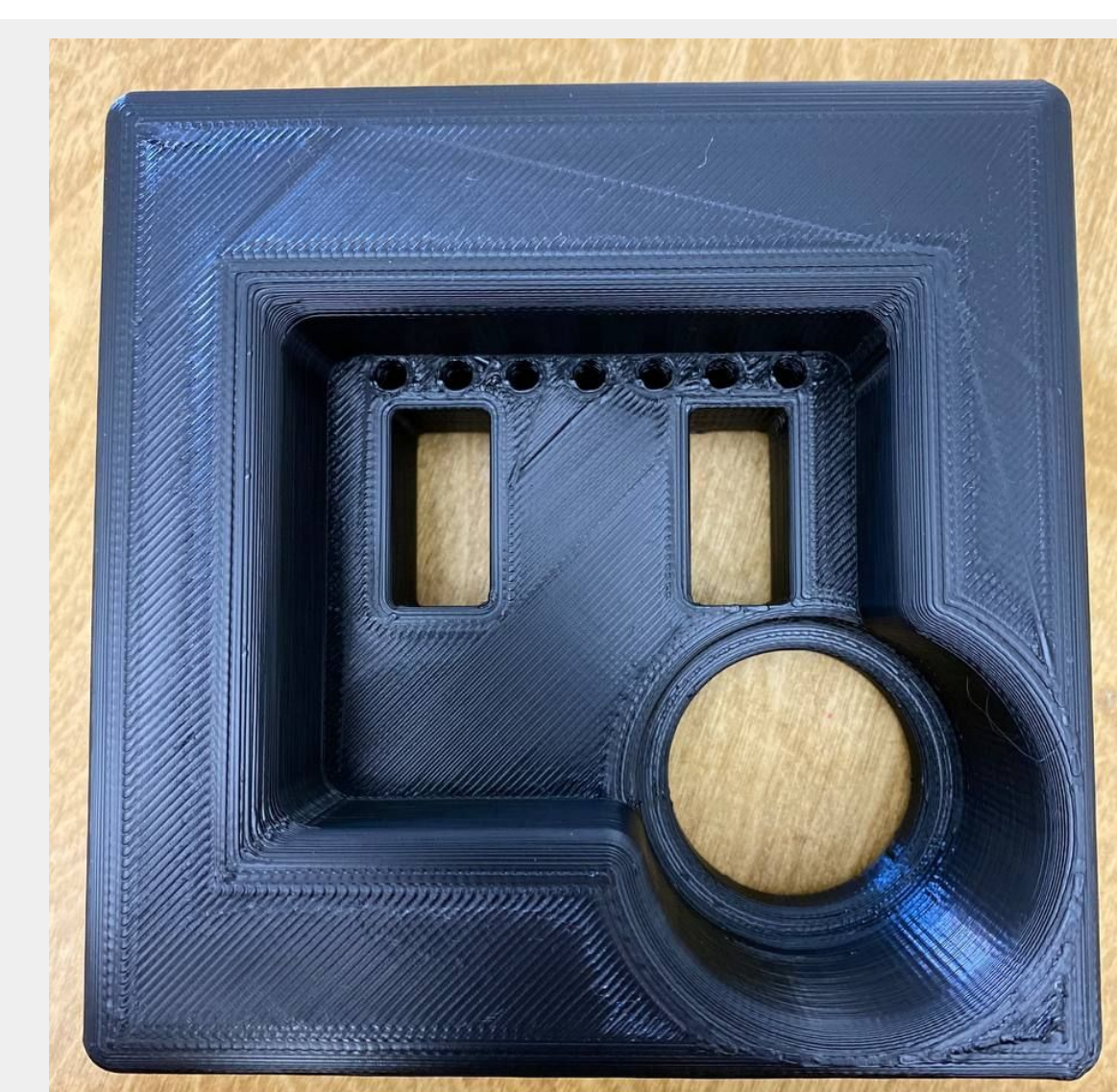
Figure 3. PCB holder with integrated slots for the excitation filter, visible LEDs, and air-cooling.
