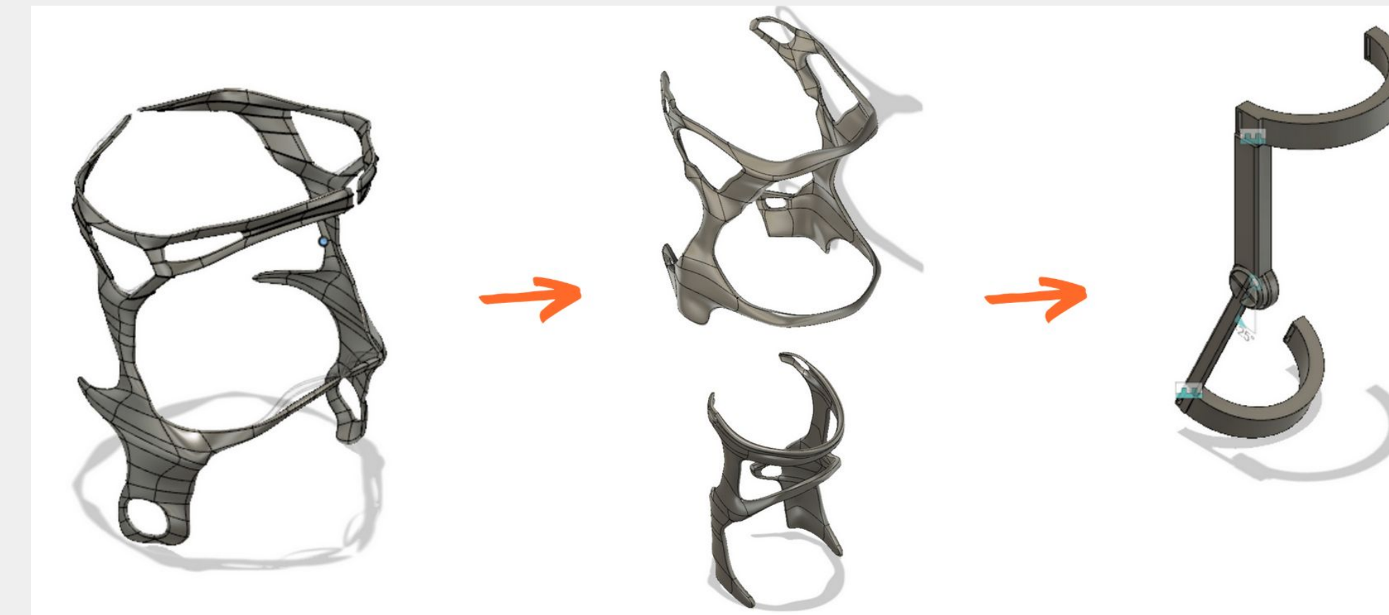
Figure 3. Brace design iterations, from original to simplified
