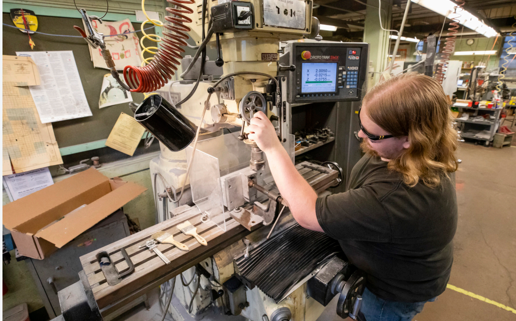
Illinois Physics lab mechanic Adam Wehe machines an EMCal block. Wehe machined over 4,500 blocks throughout the project. Photos by L. Brian Stauffer, University of Illinois Urbana-Champaign
