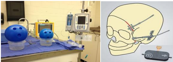
Fig.2. Growing skull models with 38 cm and 48 cm circumferences. A typical monitoring system and fluid pump from the hospital are used. The skull drawing on the right shows the concept of cranial distraction to enlarge the cranium and lower ICP. The mP6 micropump is located in the lower right corner; our plan is to reverse flow in catheters to prevent and open occluded catheters.
