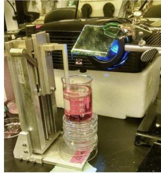
Simple SLA setup for rapid fabrication of heart models
