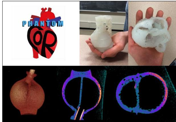
A prototype of the dynamic multimodal cardiac phantom is currently being tested using PET/CT, MRI, and ultrasound modalities. Future developments will include design and construction of 3D printed cardiac phantoms based on the collection of digital scans of pathologic human anatomic hearts available through NIH 3D Heart Library and OSF Peoria.
