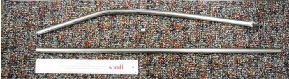
Recovered sections of 5/8" stainless steel tube
