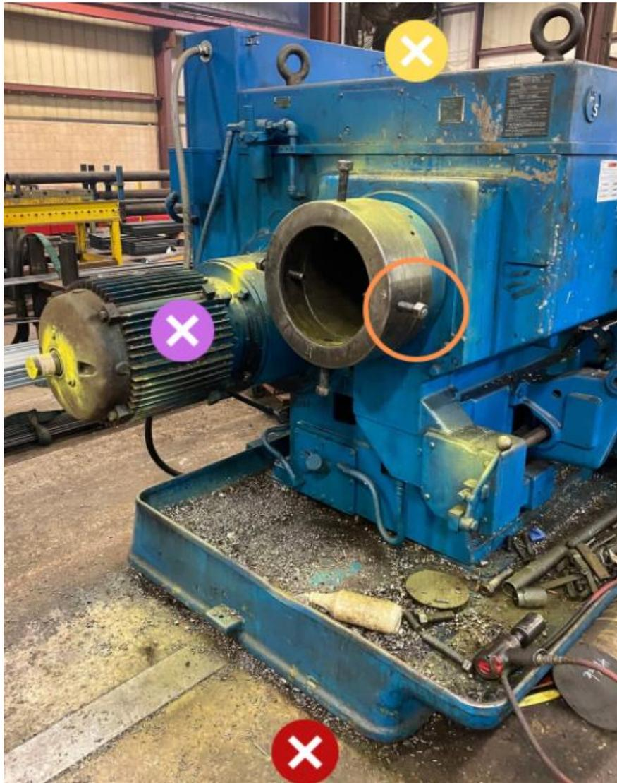
Photo 5. The **red X** indicates the position of the victim when he attempted to reach on top of the machine. The **yellow X** indicates the location believed to be where the glove was located. The **purple X** represents the lathe motor which the victim struck multiple times after becoming entangled. The **orange circle** is highlighting the chuck which caught the victim's clothing. Photo is property of KY FACE.
