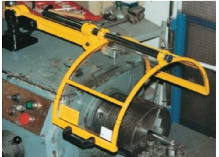
Photo 6, 7, 8 & 9. Examples of aftermarket guarding systems on similar machines.<sup>4</sup> Photos obtained from <https://www.eputec.de/en/safety-guards/safety-guards-for-lathes/>
