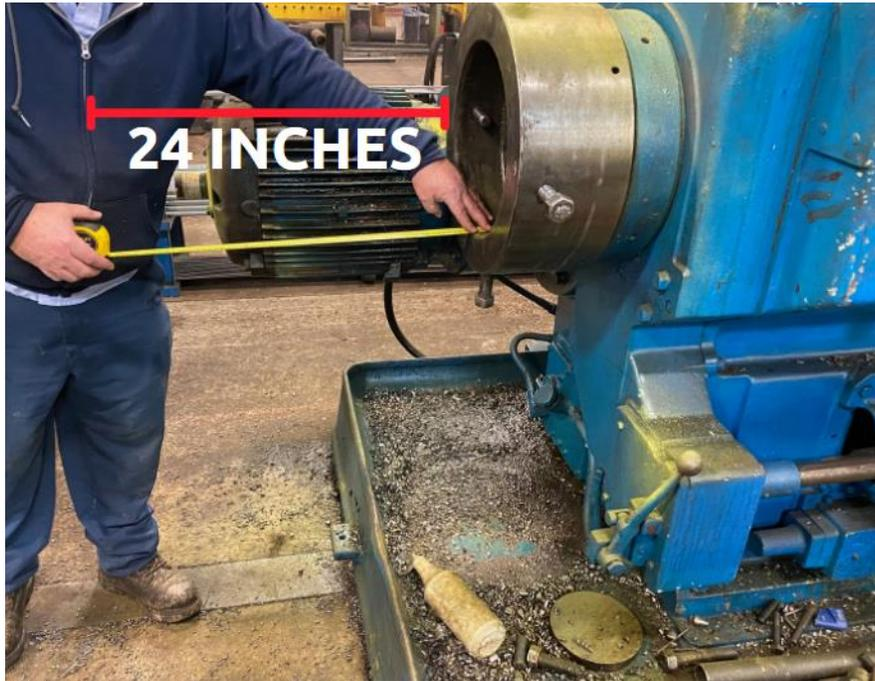
Photo 3. Photo showing the involved manual lathe. The steel rod protruded from the rear of the machine approximately 24 inches. The red line depicts how far the steel was protruding from the end of the lathe. Photo is property of KY FACE.
