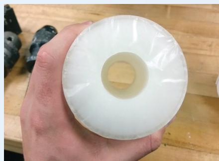
Paraffin wax fuel grain, when used with Nytrox, powers the hybrid engine.
