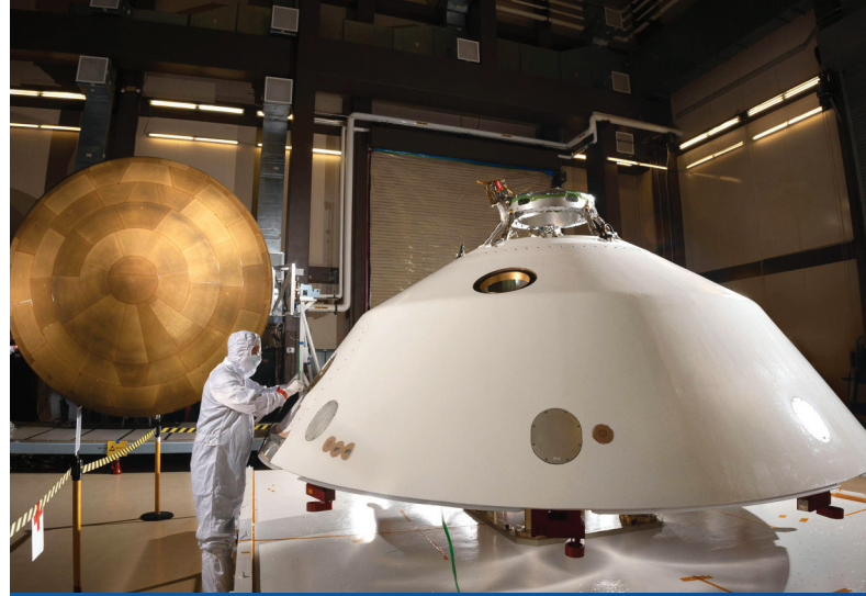
The heat shield (left) and back shell (right) comprise the aeroshell for NASA's Mars 2020 mission. Credit: NASA.
