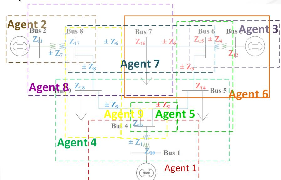
Injection: Inject false data *a* into the system by selecting an arbitrary vector *c* = [0 - 1 2 0 0 0 0 0]<sup>T</sup>
