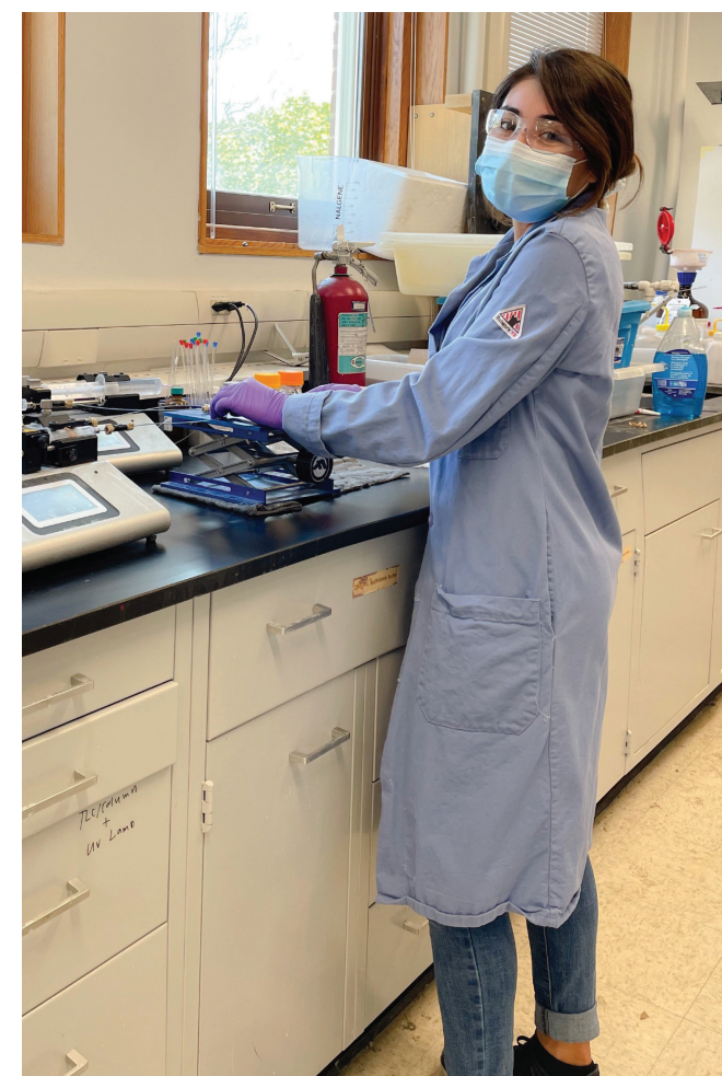
Danielle Harrier operating the droplet-based microfluidic device she designed and optimized in the Guironnet Lab. She has recently reported a water-sensitive catalyst encapsulation yielding biodegradable polymer particles dispersed in water.
