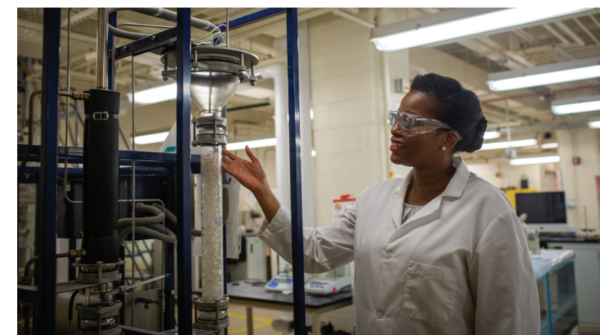
Teaching assistant professor Uzoma Monye inspects the liquid-liquid extraction column that students use to investigate the removal of t-butyl alcohol from mineral oil.
