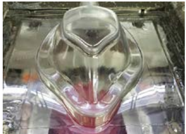
Above: Plastic mold for a prototype of the N95 mask fabrication.
