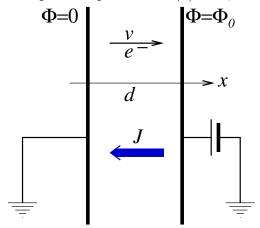
Assume that electrons (mass m, charge q = -e) are liberated at rest (v = 0) at the cathode, and are then accelerated toward the anode where they are absorbed. The charge density  $\rho(x)$  and the x component v(x) of the electron velocity do not depend on y or z. The system is in a steady state.
