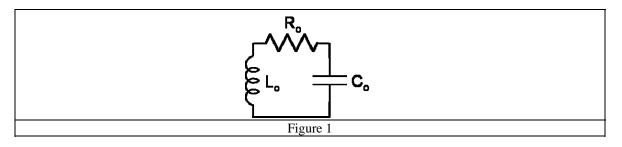
(b) Making the approximation  $\sqrt{1/L_o C_o} \gg R_o/2L_o$ , find the angular frequency of the oscillating voltage on the capacitor.
