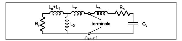
Let  $Z_o$  represent the complex impedance of the circuit elements to the right of the terminals in Figure 4, and let  $Z_k$  represent the circuit elements to the left of the terminals in Figure 4. The circuit shown in Figure 5 below is an equivalent circuit to the one shown in Figure 4.
