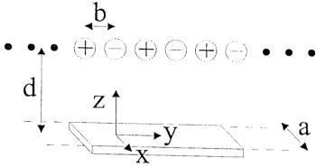
The spacing between the charges is b, and their distance from the conductor is d. The strip of conductor is given a width  $a \ll d$ .
