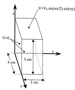
The box's 4 cm edges are parallel to the x axis, while its 3 cm and 5 cm edges are parallel the y and z axes, respectively. Five of its sides are grounded, while the top, at z = 5 cm, is held at a voltage
