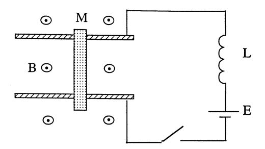
A conducting rod of mass M is free to slide without friction on two long parallel conducting rails separated by a distance D. The rails are connected through a switch to a battery of emf E and a coil of inductance L. The rod completes the circuit. There is negligible electrical resistance. A uniform magnetic field B is normal to the plane of the paper, as shown.
