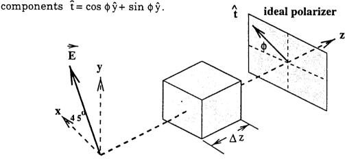
(a) The thickness of the slab ( $\Delta z$ ) is chosen to form a quarter wave plate for light with a frequency of  $\omega_o$ . This means the emerging light's  $E_y$  component is phase advanced over its  $E_x$  component by  $\pm \pi/2$ . Obtain an expression for  $\Delta z$  in terms of  $\omega_o$ , the two refractive indices, and physical constants.
