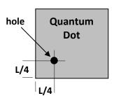
A scanning electron microscope (SEM) is used to drill a hole in the dot, at the location shown in the figure (left).
