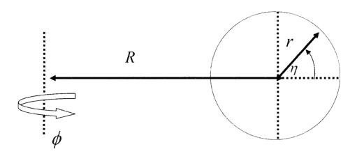
An electron of mass  $\mu$  is constrained to lie on a torus (the surface of a donut) with the dimensions depicted above. The torus is the surface that is swept out as the circle is rotated about the indicated axis as  $\phi$  is varied from  $0 \to 2\pi$ . The potential is zero when the electron is on the torus, and infinite when it is off of the torus. In the limit where
