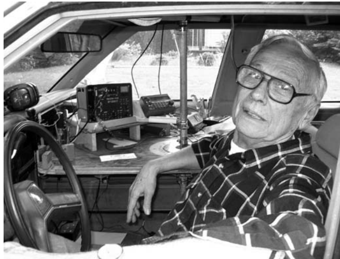
ECE alumnus Bill Cochran takes the wheel of his 1982 Chevy Caprice station wagon equipped with electronics for animal tracking. The vertical shaft connects to an overhead direction finding antenna, which tends to attract the attention of police as Cochran drives country roads in pursuit of birds.
