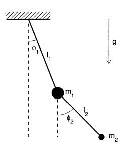
A double pendulum consists of one pendulum attached to another. Consider a double bob pendulum with masses  $m_1 = M$  and  $m_2 = m$  attached by rigid massless wires of length  $l_1 = l_2 = l$ . Further, let the angles the two wires make with the vertical be denoted  $\phi_1$  and  $\phi_2$ , as illustrated above. Finally, let the acceleration due to gravity be g. The motion is in the x-y plane and frictionless.
