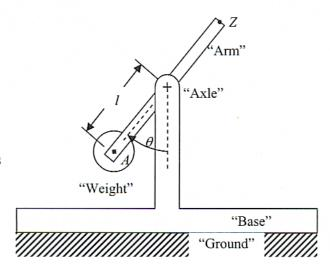
The arm is a rod of mass m, length 2l and negligible width. The weight is a disk of mass M, and radius R. The base has mass  $M_B$ .
