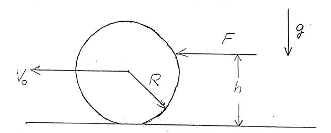
A billiard ball of mass M and a radius R is at rest on a billiard table. It is hit and given a sharp impulse (=  $\int F dt$ ) due to a very large force F acting over a very short time. The impulse is horizontally directed and at a distance h above the surface of the table. The coefficient for kinetic friction between the ball and the table is  $\mu$ . Note that the moment of inertia for a billiard ball about its center is  $2M R^2/5$ .
