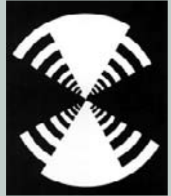
Diagram of DuHamel’s toothed bowtie design.
