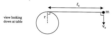
The string remains taut and proceeds to wind around the peg as the mass slides without friction on the table. After a short time some of the string has wound up and the system looks like:
