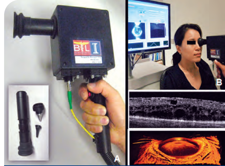
An early prototype of the handheld scanner has both OCT and video-imaging capabilities and interchangeable tips for the eyes, ears, skin, and oral tissue. As one example, the device images the retina and the anterior eye structures (bottom right).
