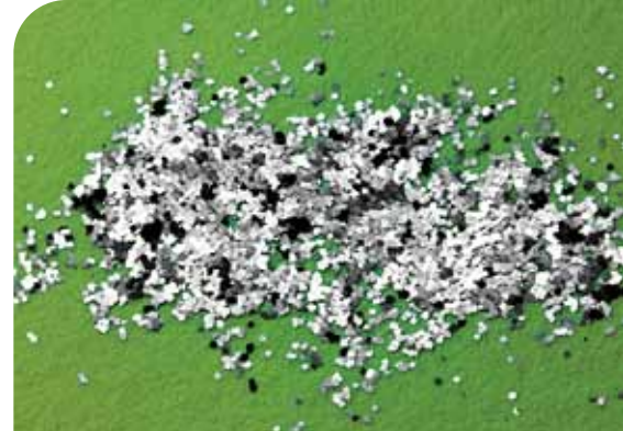
A pile of gallium arsenide solar cells manufactured in stacks and then peeled apart layer by layer. They can be integrated into a number of electronic devices. Photo courtesy John Rogers
