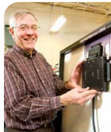
ECE Professor Philip Krein demonstrates how one of SolarBridge's devices attaches to a photovoltaic board.
