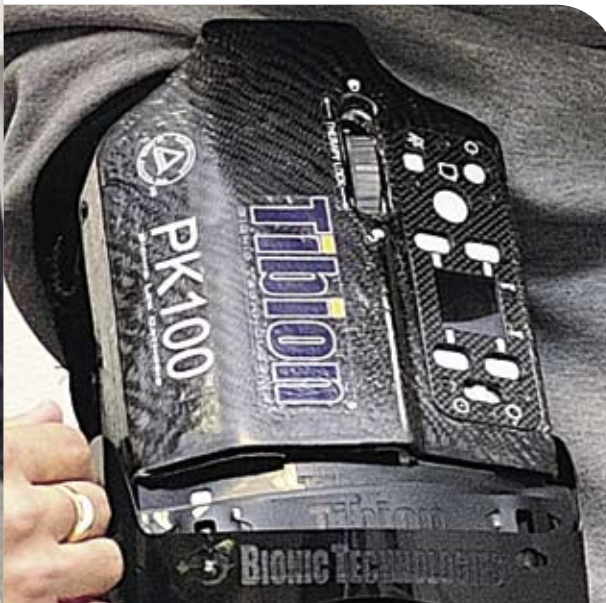
The Tibion PK100 is a powered, assistive leg device that enhances knee rehabilitation therapy. Photo courtesy of Robert Horst.
