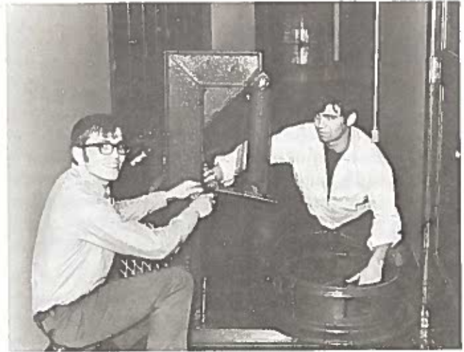
Truck Tire Changer. Award-winning duo Mike Cleary (left) and Jerry Wagner demonstrate their prototype. This equipment is adjustable for tire sizes from 16" to 22" rims, yet it is priced less than half the cost of currently available equipment.
