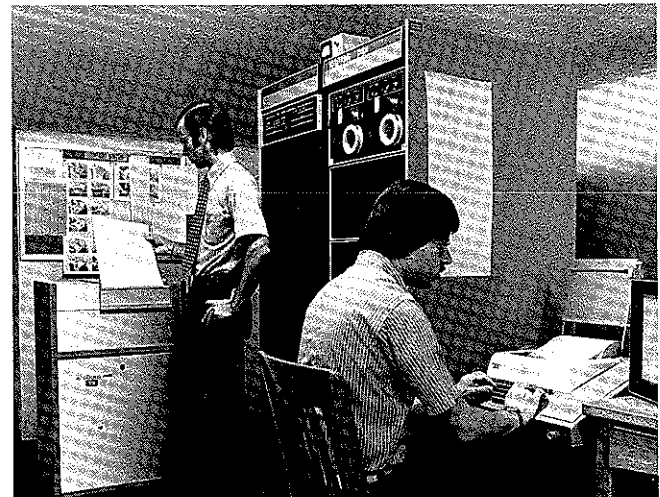
Professor M. H. Pleck (standing) and graduate student D. D. Burn test a new line printer driver for the PDP-11/20-Gould 800 electrostatic raster plotter. This driver was an integral part of the engineering graphics program being developed on minicomputers in 1974.
