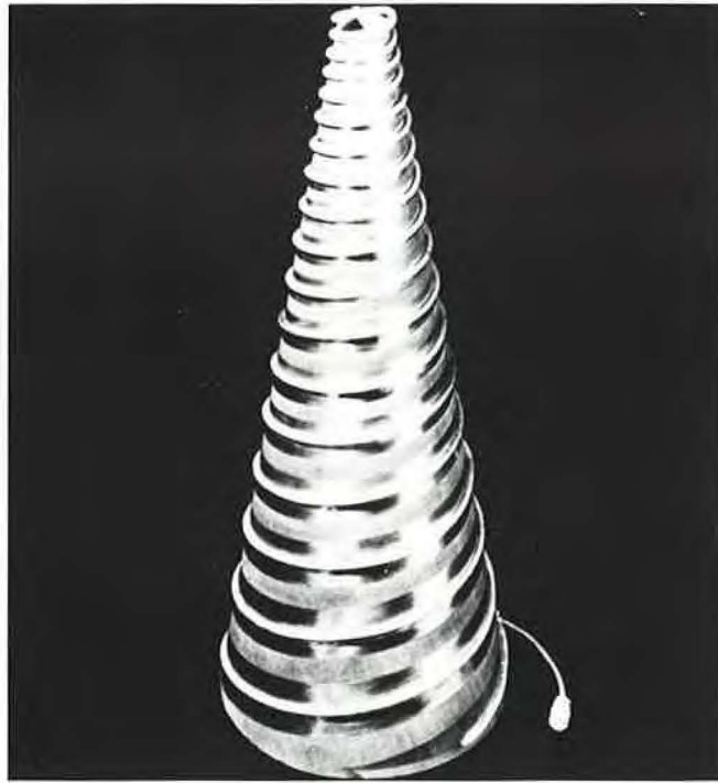
Spirals on a conical shaped unidirectional antenna.
