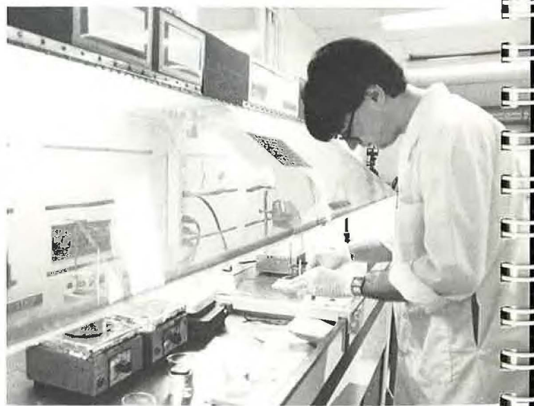
Students enrolled in E.C.E. 344 make transistors. They must clean the wafer's surface with acids and solvents because device geometries are comparable to the size of a dust particle.
