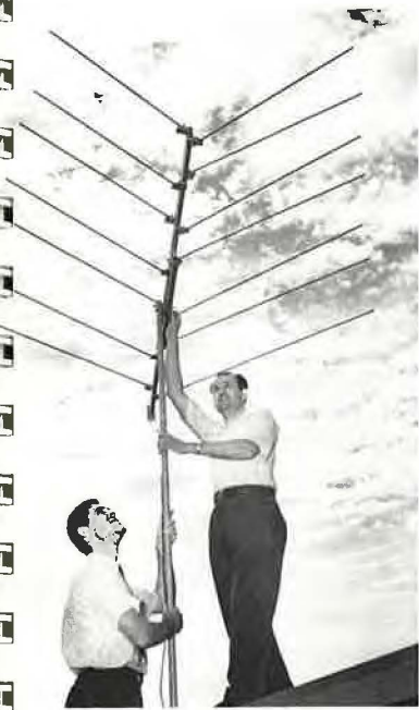
Paul Mayes (right) and Robert Carrel developed the log-periodic antenna. It became the most popular antenna for television reception and is one example of a by-product from military research conducted at the university
