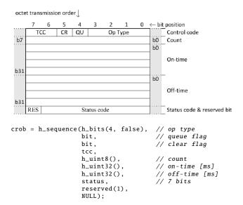
Figure 5: The DNP3 CROB object (IEEE 1815-2012) and the Hammer-based code for handling it.
