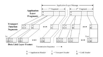
Figure 1: DNP3 protocol layers (Fig. 0-2 in IEEE 1815-2012)
