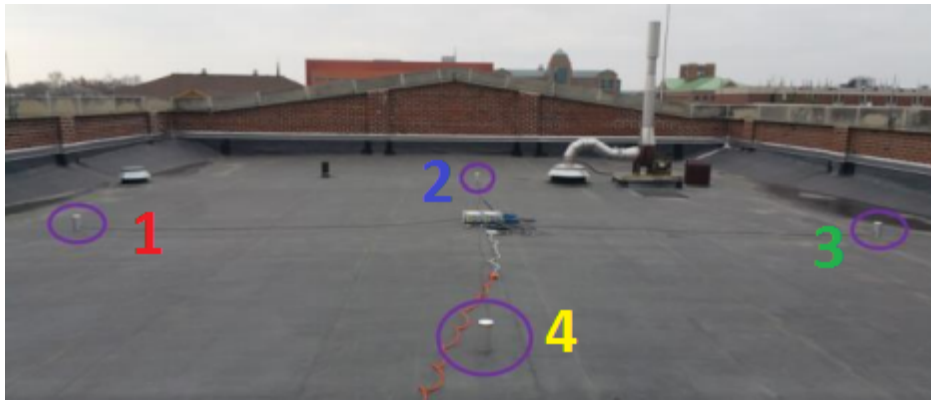
Figure 4.1: Four GPS antennas located on roof of Talbot Laboratory, University of Illinois at Urbana-Champaign (UIUC). Reference image taken from [23].
