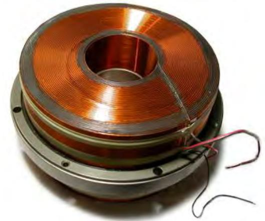
We can change the strength of the lens (i.e. the focal plane) by changing the current, but not the shape of the fields.
