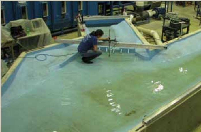
Christiana Barnas sets up a Vectrino probe to take flow velocity measurements just downstream of the dam. She will leave the basin and go to the computer, which is connected to the probe, and start collecting data. The probe collects flow velocity data for 1-2 minutes. This is repeated for 50 points in a given cross-section. For each point, a time-averaged flow velocity is computed. This shows the velocity distribution in a given cross-section.
