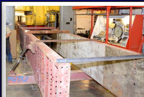
Failure testing of girder-plate beam Displacement, strain measurements in 3-point bending
