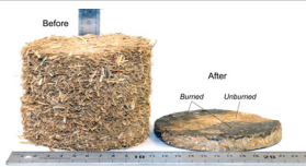
High-pressure compaction of biomass—switchgrass and miscanthus Compression to 110,000 psi in one miscanthus sample caused self-ignition
