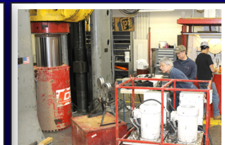
Hydraulic ram calibration to 3 million lb Traceability to NIST is critical for construction industry
