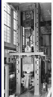
Riveted joint tests, ~1950 Nathan Newmark, William Munse
