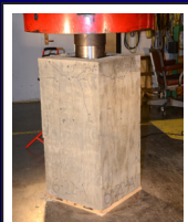
Cable anchor testing Progressive failure monitoring
