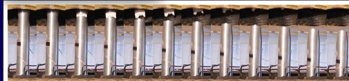
Dynamic tensile failure of 6061-T6 aluminum, TAM 252 High-speed images (300 frames/s) of 5-in.-dia. bar immediately after failure at 1 million lb
