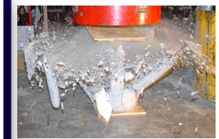
Crushing of concrete cylinders at EOH Failure load of 18-in.-dia. cylinders approaches 2 million lb
