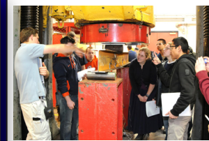
Plastic deformation of I-beam, TAM 456 Students use electrical-resistance strain gages to analyze stress
