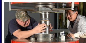
High-pressure compaction of biomass—switchgrass and miscanthus Compression to 110,000 psi in one miscanthus sample caused self-ignition
