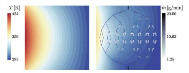
Computational design of microvascular materials. Generalized finite element analysis of the effect of a microvascular network on the thermal field in a square polymeric component. Left: Temperature field in the absence of flow. Right: Thermal solution obtained for a hierarchical network with a 20 g/min mass flow rate of cooling fluid.
