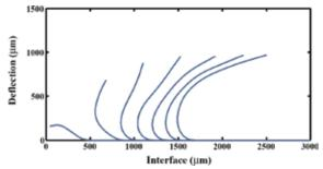
Laser-induced delamination of thin films. (left) Laserinduced delamination of aluminum film on silicon substrate. (above) Numerical simulation based on dynamic nonlinear beam model
