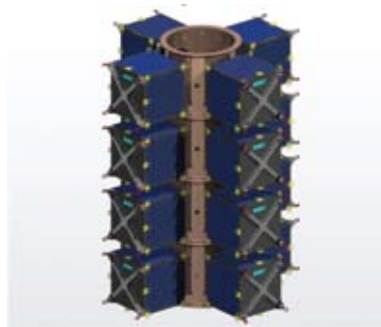
All 16 ADIOS Spacecraft arrayed before separation
