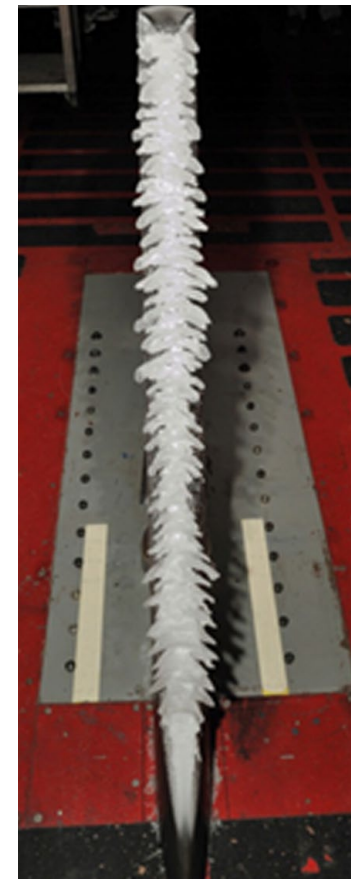
Photograph of swept wing ice accretion produced in NASA's Icing Research Tunnel
