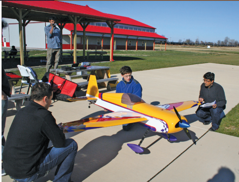
Graduate students, Adam Ragheb, Pritam Sukumar, Or Dantsker, and Gavin Ananda checking balance on the 35%-scale aerobatic Extra 260 before conducting spin tests at Eli Field in Monticello, IL.
