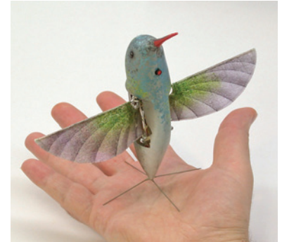
AeroVironment Nano Hummingbird named one of the “50 Best Inventions of 2011” by TIME Magazine. UIUC’s involvement included water channel testing airfoils at very low Reynolds numbers. Photo: Wikimedia Commons
