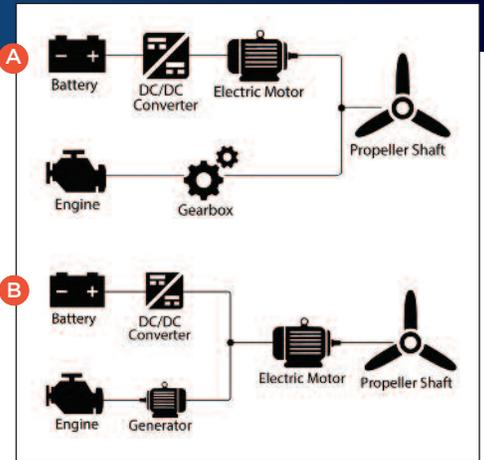
This figure shows the a) parallel and b) series drivetrain models.
